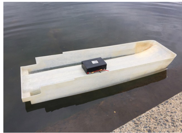
Left: USNS Spearhead (JHSV-1) Right: Displacement testing the hull.
