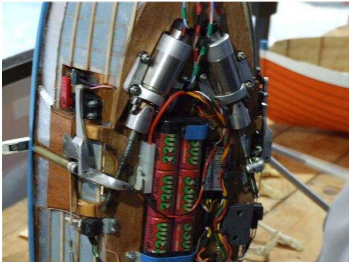
The inner shell of the Skeleton Rowboat removed, to show the clever way the electronics and mechanicals are installed out of view. Each oar is independently controllable in speed and direction. You can see the orange outer shell in the background.
